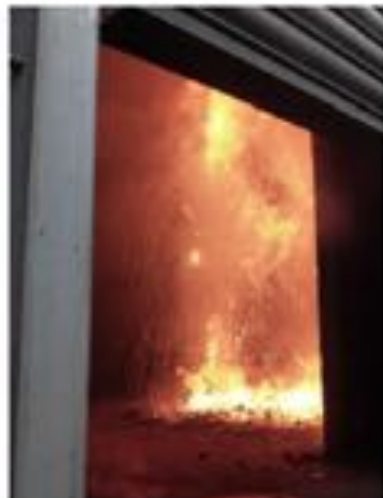
Figure 6 - PIR insulated system with PE ACM panels (note test had to be stopped early, after 12 minutes)
