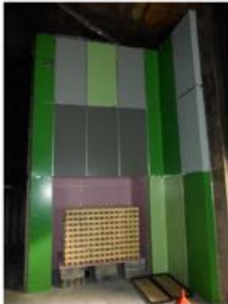
Figure 5 - Phenolic insulated system with A2 ACM panels
