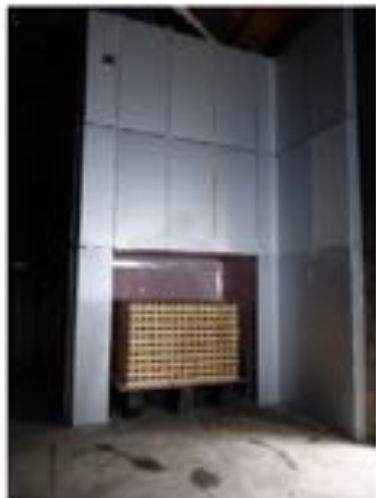
Figure 6 - PIR insulated system with PE ACM panels (note test had to be stopped early, after 12 minutes)
