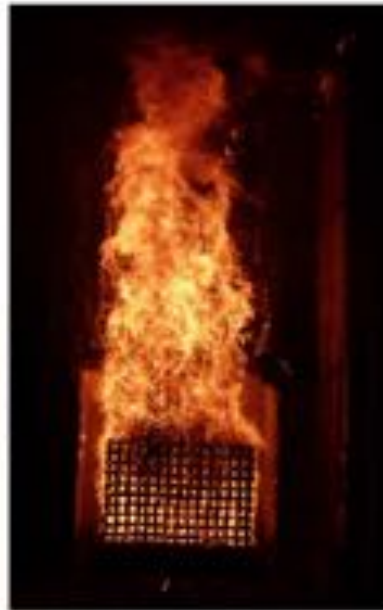
Figure 5 - Phenolic insulated system with A2 ACM panels
